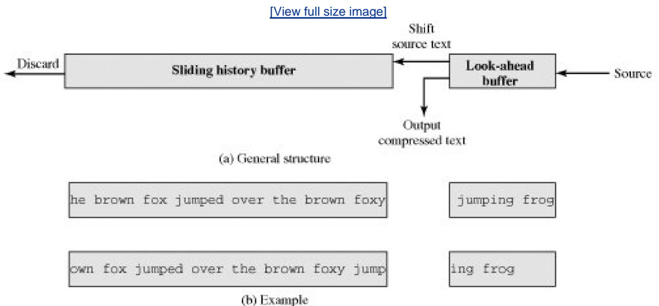
[Figure 15.10b](#) shows the operation of this scheme on our example sequence. The illustration assumes a 39-character sliding window and a 13-character look-ahead buffer. In the upper part of the example, the first 40 characters have been processed and the uncompressed
