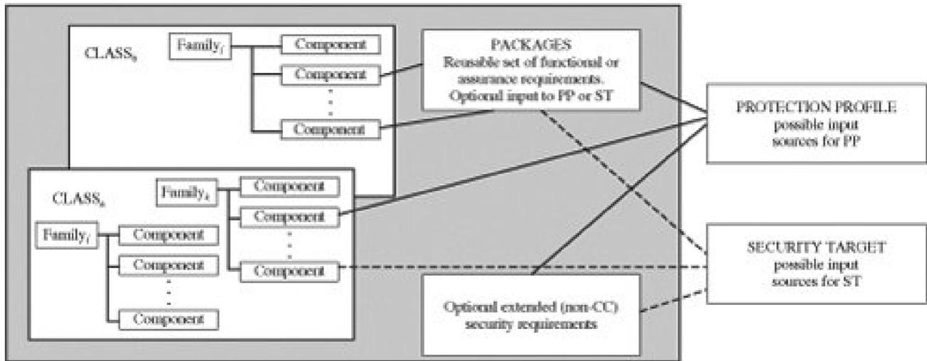
[Figure 20.7](#) shows what is referred to in the CC documents as the security functional requirements paradigm. In essence, this illustration is based on the reference monitor concept but makes use of the terminology and design philosophy of the CC.
