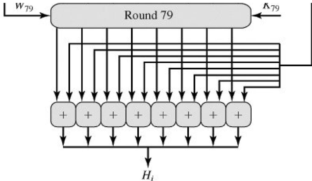
Each round takes as input the 512-bit buffer value  $abcdefgh$ , and updates the contents of the buffer. At input to the first round, the buffer has the value of the intermediate hash value,  $H_{i-1}$ . Each round  $t$  makes use of a 64-bit value  $W_t$  derived from the current 1024-bit block being processed ( $M_i$ ). These values are derived using a message schedule described subsequently.
