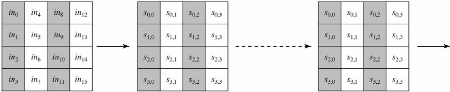
(a) Input, state array, and output
