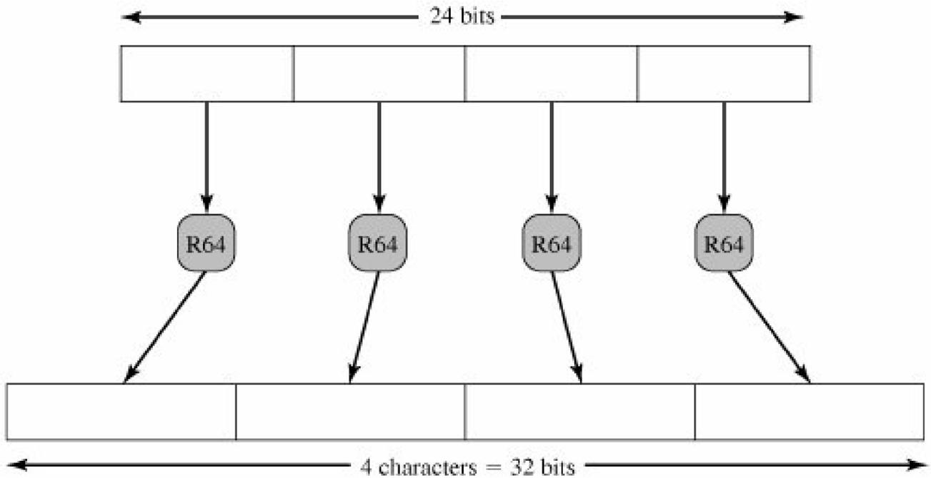
For example, consider the 24-bit raw text sequence 00100011 01011100 10010001, which can be expressed in hexadecimal as 235C91. We arrange this input in blocks of 6 bits:
