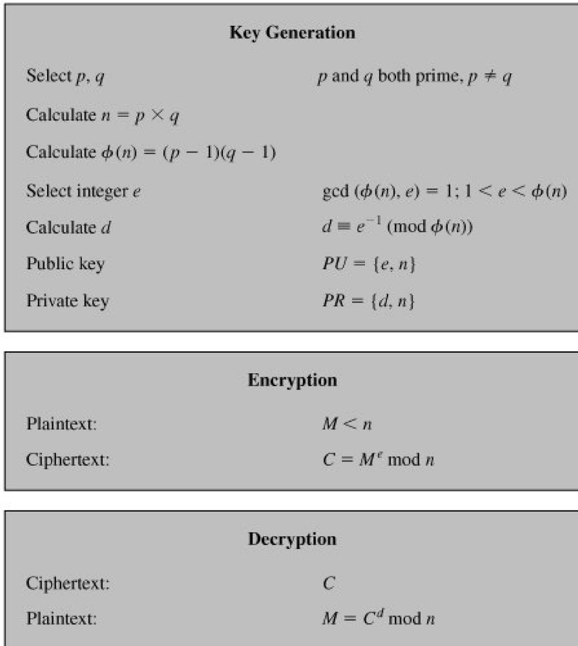
Figure 9.6. Example of RSA Algorithm
